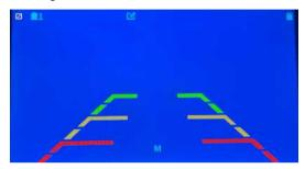
Press the 'OK' button three times when 'W' appears in the center of the monitor to adjust the width of the guideline. Use the '+' button to widen it and the '-' button to narrow it.
