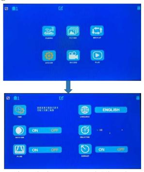
After entering the menu page, press the '+' button three times and then press 'OK' to access the TIME, LANGUAGE, AUTO-DIM, DELAYTIME, P-LINE, and DEFAULT settings.
