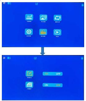
After entering the menu page, press the '+' button four times, then select 'RECORD,' and press 'OK' to access the RECORD settings.
