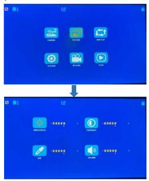
Press the 'M' button to enter the menu page, then press the '+' button, and finally press the 'OK' button to access the Picture menu, where you can adjust the monitor's brightness,
