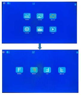
After entering the menu page, press the '+' button twice and then press 'OK' to access the settings page. Make your desired adjustments, and once they are complete, press 'OK' to confirm. Press the 'M' button to go back.
