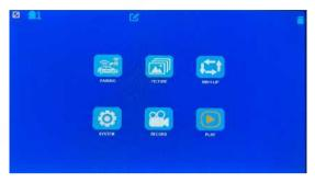
After entering the menu page, press the 'M' button to access the menu, then press the '+' button five times (or once after entering the menu '-') to select 'PLAY,' and confirm by pressing 'OK.' Here, you can play video files. Loop recording is supported, and it will automatically overwrite old files when the SD card storage is full.
