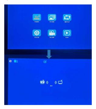
After pressing the "M" button to enter the menu page, then press the "OK" button to confirm to enter the "PAIRING" page for pairing and connecting the camera.
